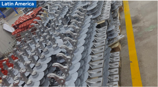
Puerto Rico | 15kV, 25kV Composite Line Post Insulators Project
